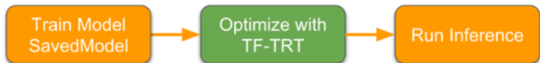
Figure 5.6: TF-TRT workflow for SavedModel format models.
