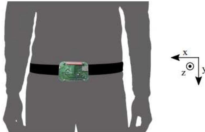
Figure 4.6: Device used for acquisition. The self-developed embedded device included two accelerometers and a gyroscope. It was fixed to the waist of the participants [51].
