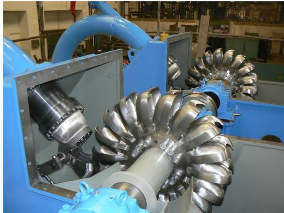
Figura 5: Turbina Pelton [18]
