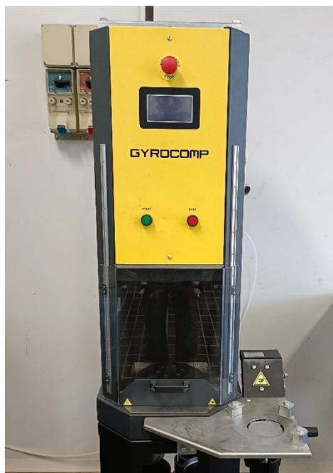
*Fig. 3.7 – Pressa giratoria Gyrocomp*
