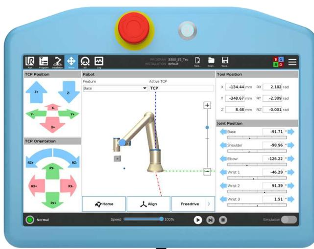
Figure 13: PolyScope
