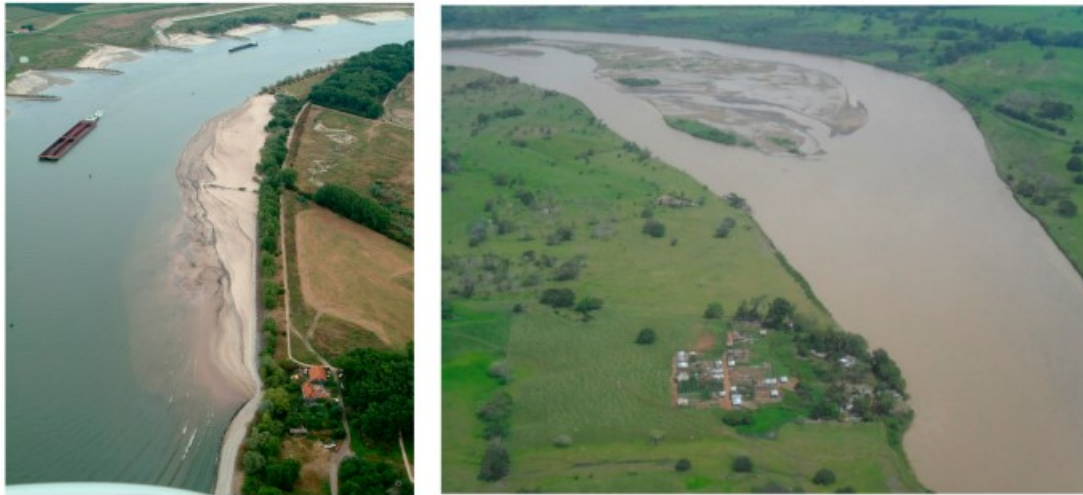
Figure 3. a) Point bar inside a river bend (Rhine River, the Netherlands). b) Compound central bar forced by a local width expansion (Cauca River, Colombia).
