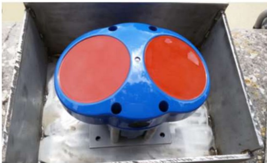
Figure 17. H-ADCP river gauge
