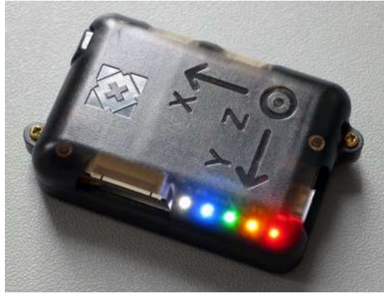
Figure 10: NGIMU box case.
