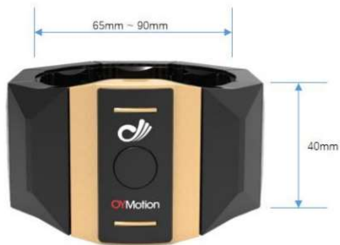
Figure 6: OYMotion GForcePro+ dimensions [28] .
