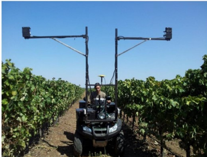
Figura 4-3 sensori prossimali multispettrali (fonte: State of the Art of Monitoring Technologies and Data Processing for Precision Viticulture, M. Ammoniaci, S. Kartsiotis, 2021)
