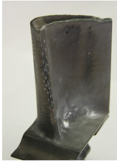
(a) Erosion of the leading edge of a gas turbine blade
