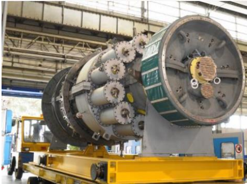
Figura 5. Gas Turbine, frame technology.
