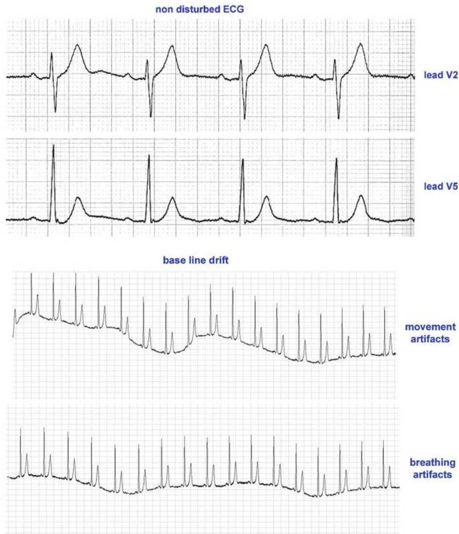
Figure 3.6: Low frequency noise present in ECG signal [34]
