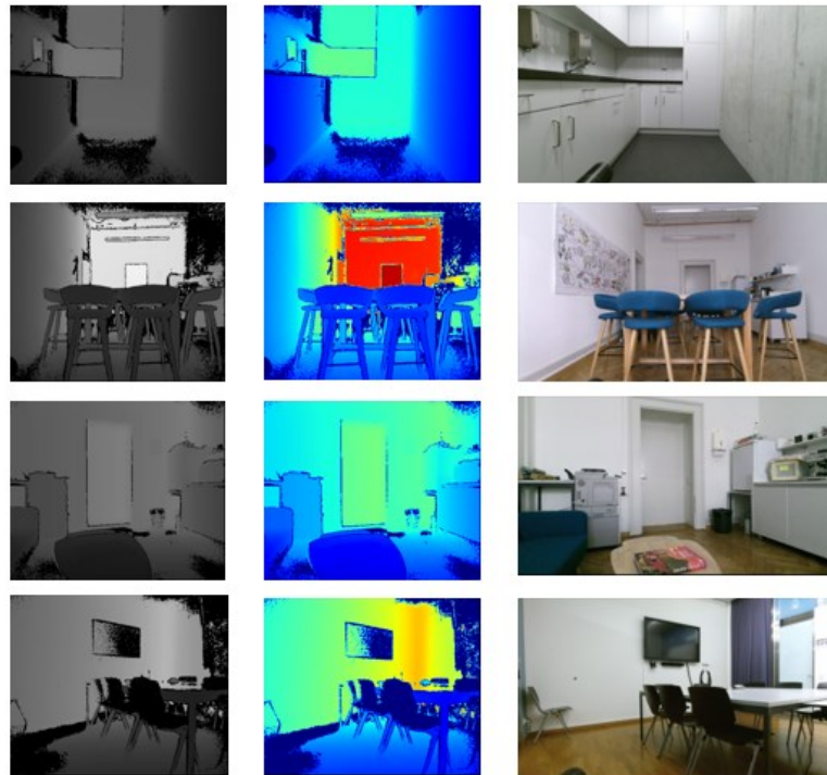
Figure 6. Examples of the Kinect samples acquired at the university. In order, grayscale depth image, depth image in jet colormap, RGB image of an apartment scenario
