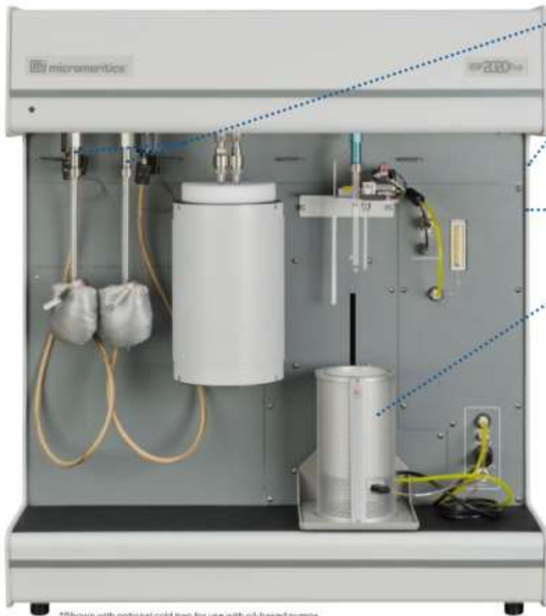
Programmable, two-station degas system allows physisorption sample preparation while running a chemisorption analysis
