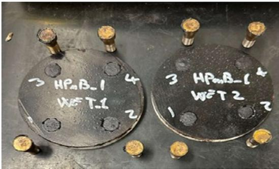
Fig. 4.59 Rotture indesiderate, aggregato calcareo
