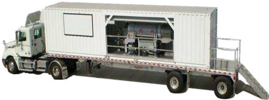
Figura 13 impianto mobile in container Mena water https://mena-water.com/container/sludge-dewatering-unit/
