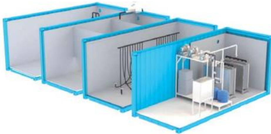
figura 18 impianto mobile in container green MBR, https://www.idro.net/upload/blocchi/MBR.pdf
