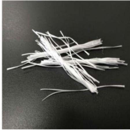
Fig. 2.6 – fibra Readymesh PF
