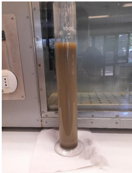
FIGURE 16 SLURRY INSIDE THE SEDIMENTATION CYLINDER
