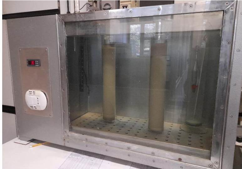
FIGURE 17 SEDIMENTATION CYLINDER INSIDE THE WATER BATH
