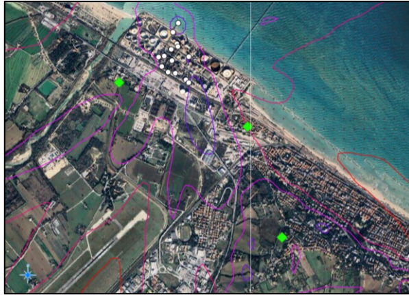
Figure 71. Monitoring station locations (green) and sources (white) visualized in QGIS over analyzed gradient lines (purple)
