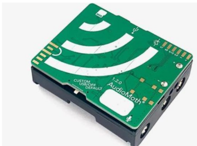
Figura 12 Bat detector AudioMoth v1.2.0 (Open Acoustic Devices).
