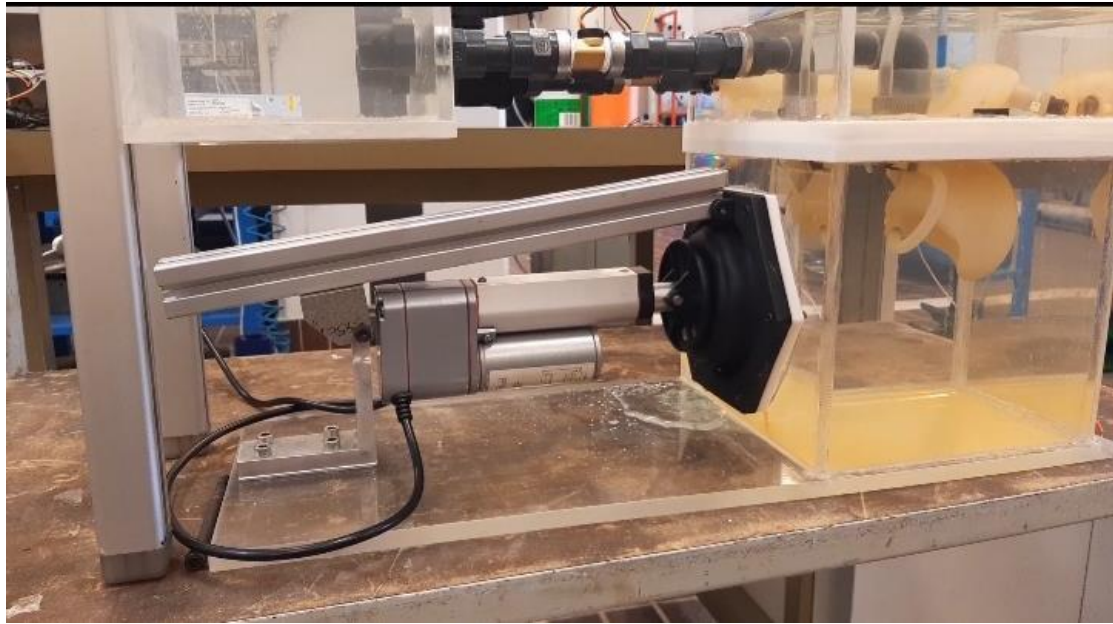
Figure 18 Realization of aortic test bench
