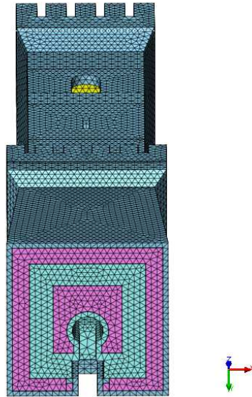
Figure 4-7 – Mock-up of the second step of calibration. The filling is represented in purple colour, while the masonry parts are in light blue.
