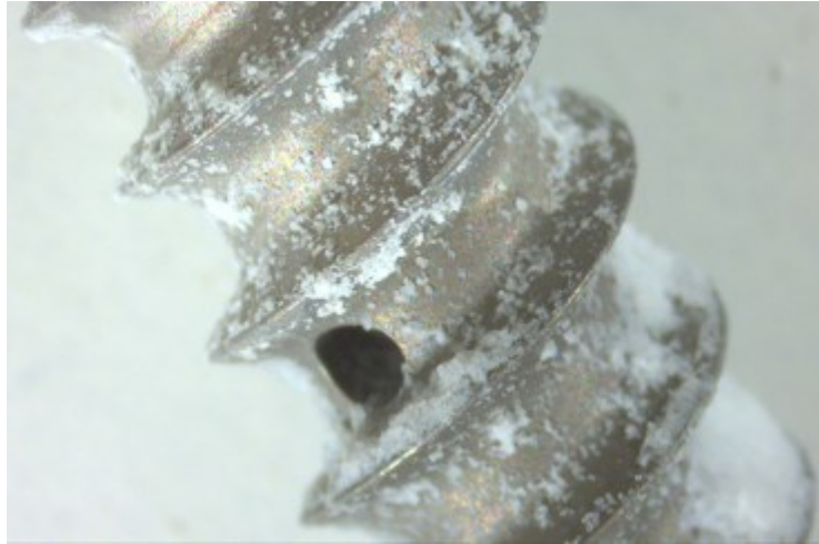
Figure 60 S082h : T > 100^{\circ}\text{C} /sprinkled with \text{HA} + \text{H}_2\text{O}_2 and heated directly on a thermal plate for 2 min.
