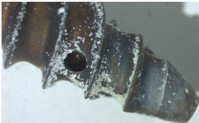
Figure 66 S362m : 100°C/ immersed in 1:2 mix (0,5g+1ml of NaOH (1,4 mg/ml)-H 2 O 2 ) for 10 min.
