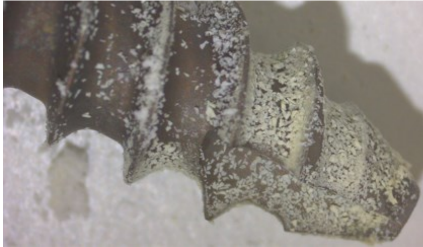
Figure 62 S656m (S928m) : 100°C/soaked in 1:2 mix (0,5g+1ml of NaOH-H 2 O 2 ) for 10 min.
