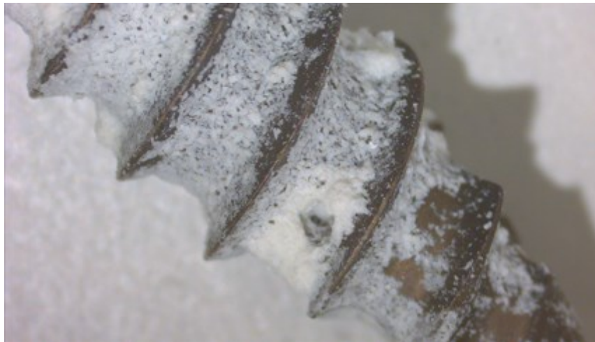
Figure 61 S398h ( S249h ): 100^{\circ}\text{C} /soaked in 1:2 mix (0,5g+1ml of \text{NaOH} - \text{H}_2\text{O}_2 ) for 10 min.
