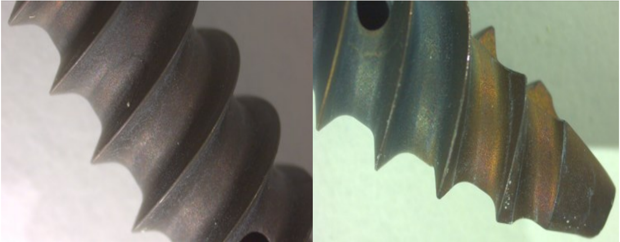
Figure 51 S133m(S459m) : 100°C/soaked in 6:10 mix for 10 min. S016h : 100°C/soaked in 6:10 mix for 10 min.
