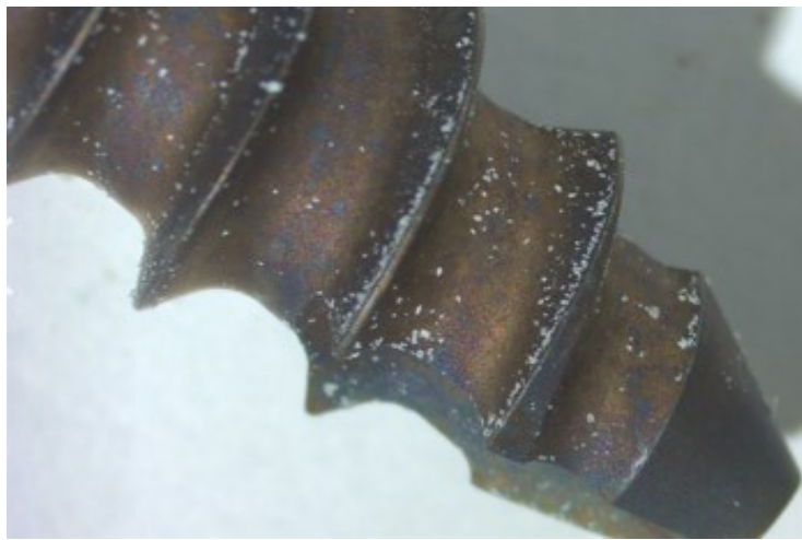
Figure 65 S909m : 100°C/ immersed in 1:2 mix (0,5g+1ml of NaOH (0,14 mg/ml)-H 2 O 2 ) for 10 min.
