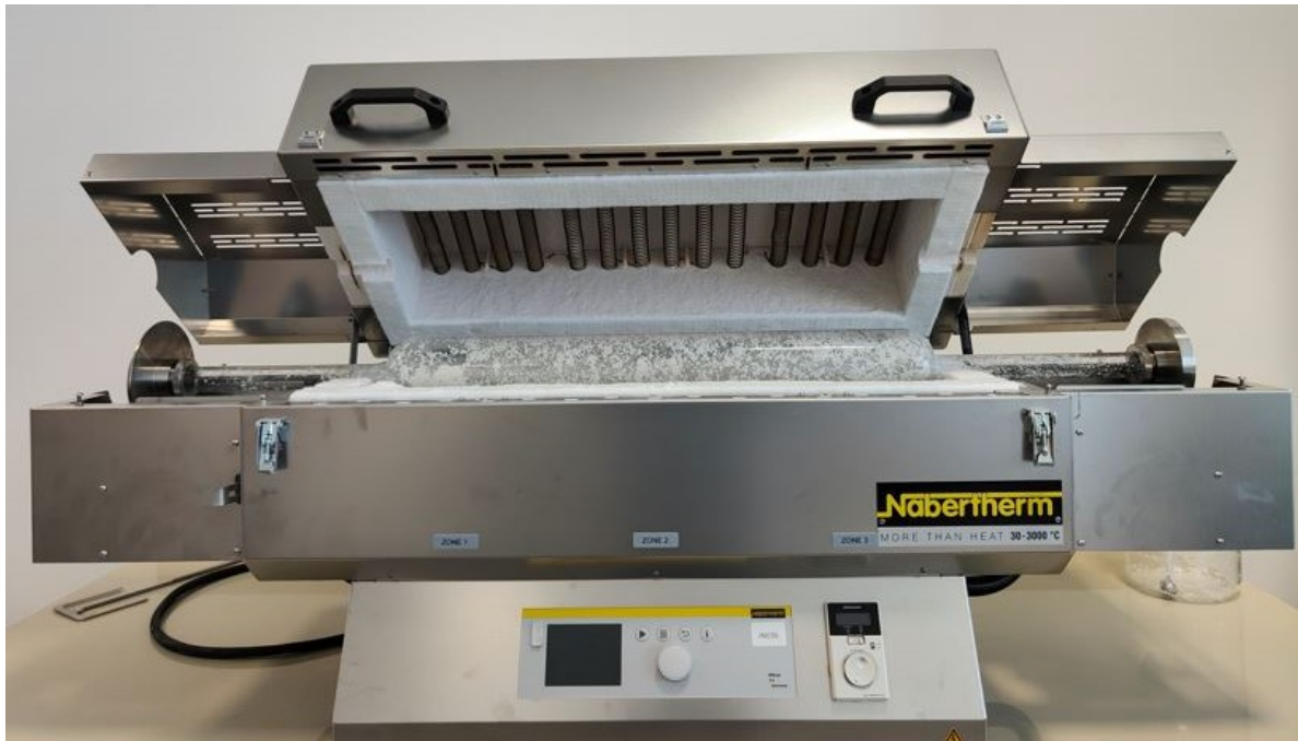
Figure 22 Nabertherm calciner loaded with the cell of calcination filled with decellularized bone powder.
