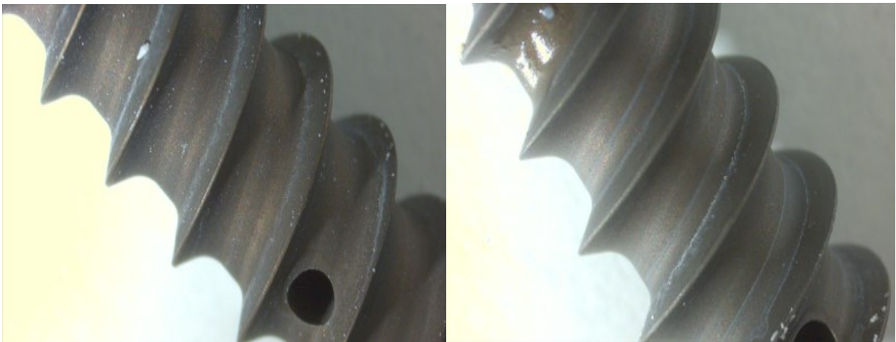
Figure 50 S876m : 100°C/soaked in 2:10 mix for 10 min. S391m : 100°C/soaked in 4:10 mix for 10 min.
