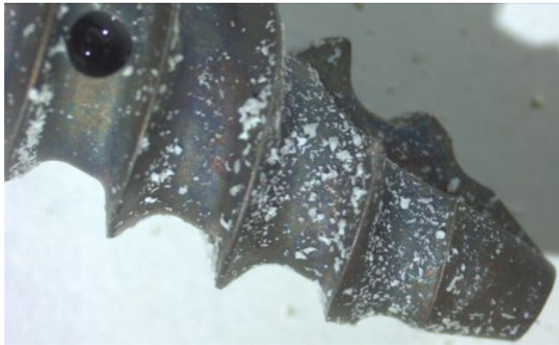
Figure 63 S329m : 100°C/sprinkled with 1:2 mix (0,5g+1ml of NaOH-H 2 O 2 ) and heated directly on a thermal plate for 2 min.
