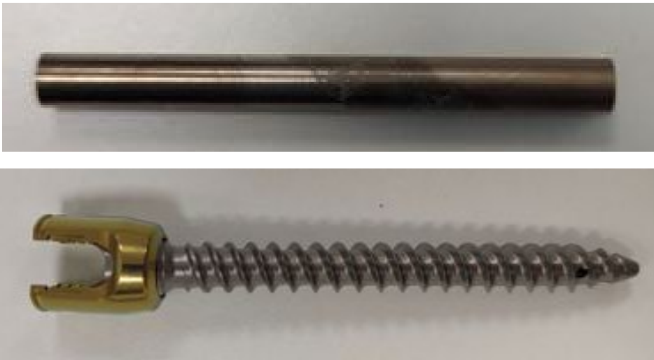
Figure 24 Grade 6 titanium bar (on top), Grade 4 titanium screw (on bottom).
