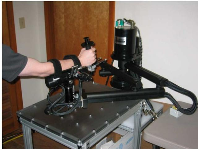
**Figure 1.3.:** MIT-Manus robot for upper limb rehabilitation [39].
