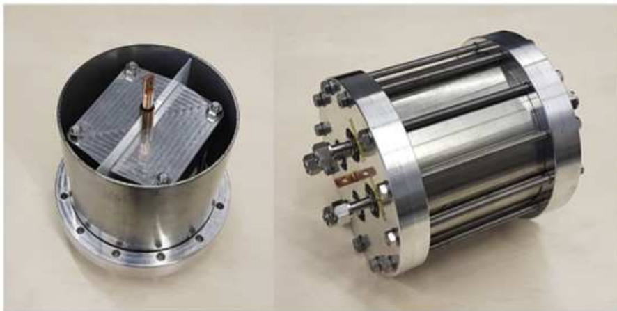
Figure 15: Photograph of the PEMEL stack with a reinforced pressure housing [51].
