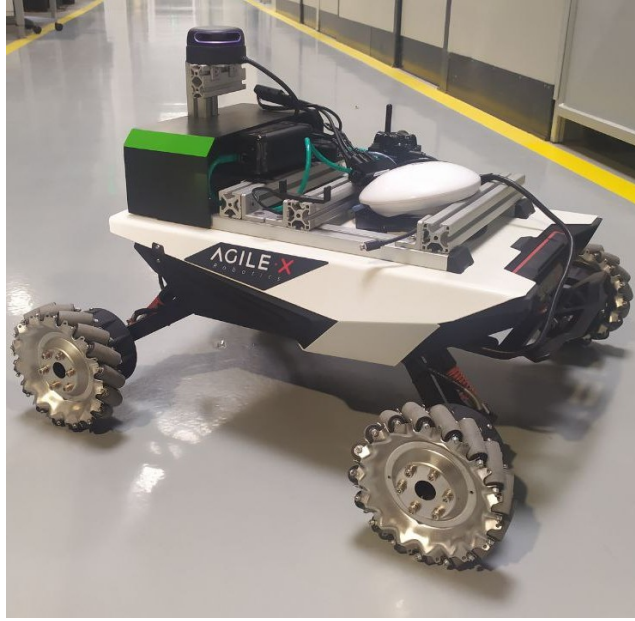
Figure 1.10: Scout Mini Robot with electronic equipment
