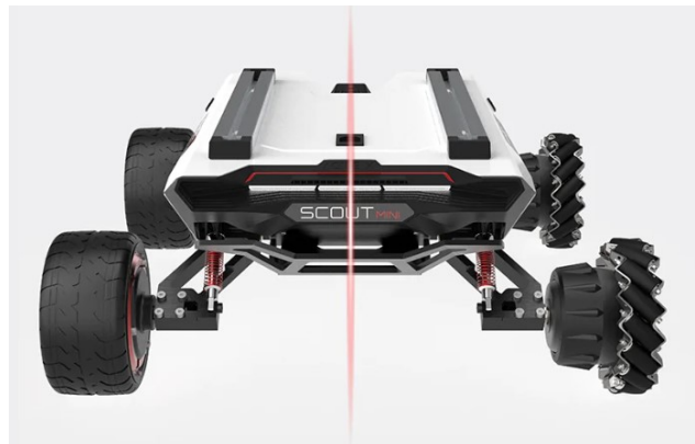
Figure 1.9: Wheel Equipment Available for Scout Mini
