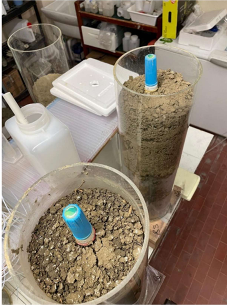
Figure 7: emplaced drill&drop Sentek probes to monitor the soil water and solutes movements.
