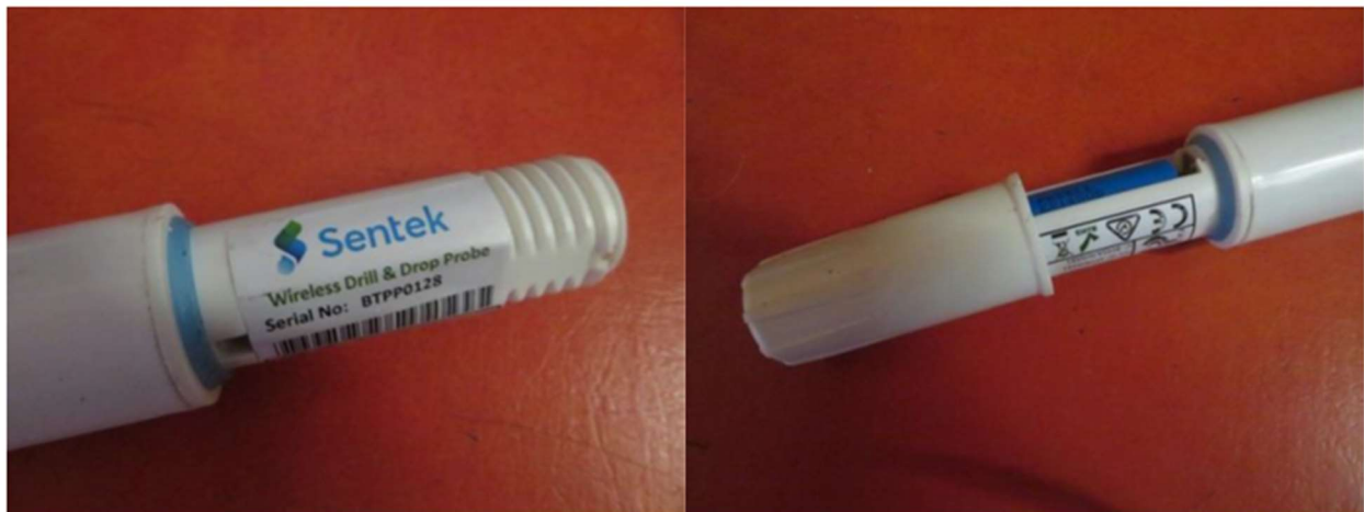
Figure 9. Bluetooth Probe head incorporating battery compartment, antenna and serial number This probe has similar functionality to other Sentek Drill & Drop Probes such as SDI-12 Series III or Sentek RS232/485 Series II probes incorporating a Sentek EnviroSCAN interface box.
