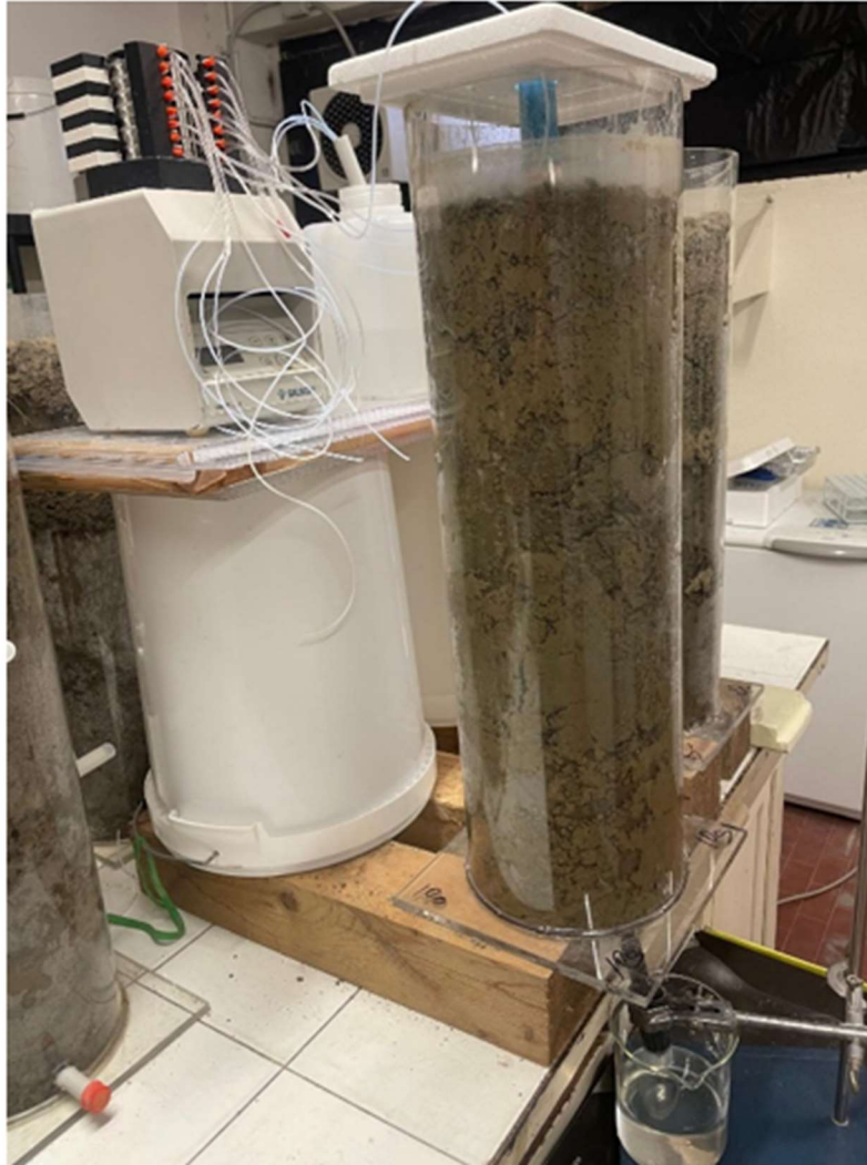
Figure 8: Experimental synthetic rainfall simulator and fraction collectors.
