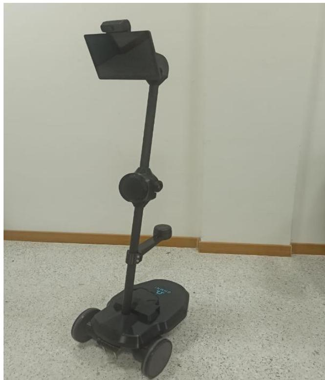
*Figura 1 Ohmni Telepresence Robot*
