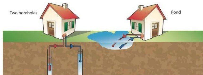
Figure 6 - Typologies of Open loop system exploiting groundwater (left) and surface water (right).
