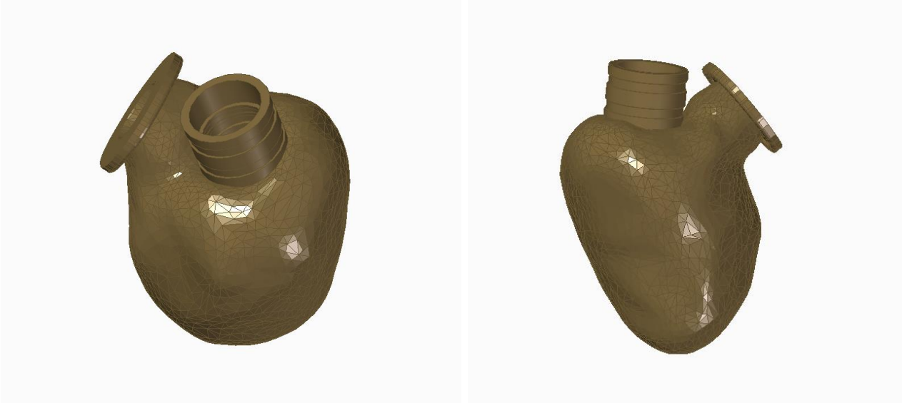
Figure 31. Left ventricle after modifications for the insertion of the valves and the tubes.
