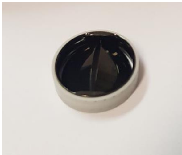
Figure 35. Mitral valve used in the present test bench.
