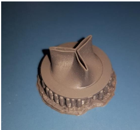
Figure 48. 3D printed aortic valve with printing supports (left) and without support (right).
