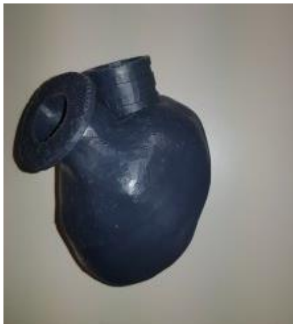
Figure 43. 3D printed left ventricle from different points of view.
