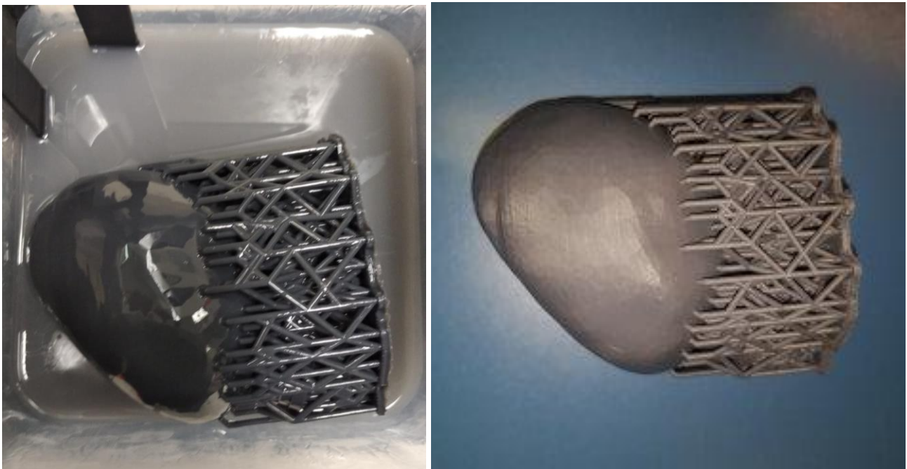
Figure 42. 3D printed Left ventricle with supports due to the Formlab printer.
