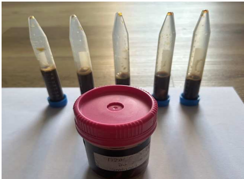
Figure 14: Staining Protocol. The specimens are immersed in a coffee solution for two weeks.
