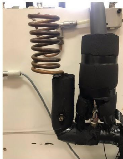
Fig. 2.10 Serpentina in rame esterna
