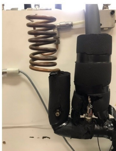
Fig. 2.10 Serpentina in rame esterna
