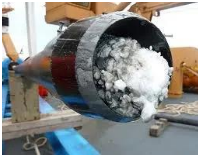
Figure 36: Hydrate Formation in the Gas Stream. Gas Hydrates
