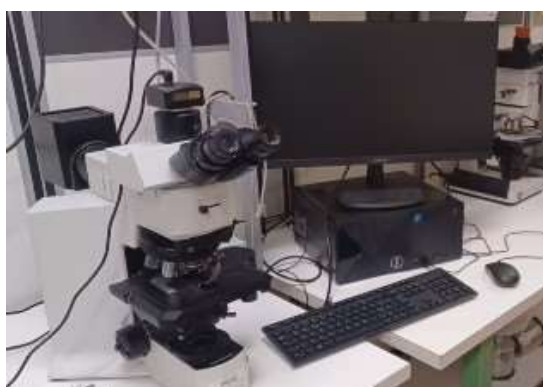
Fig.27: Olympus BX-51 fluorescence microscope for blend analysis
