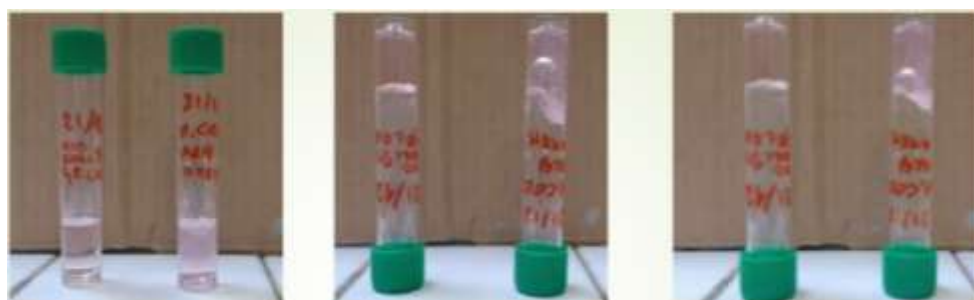
Fig.41: Collagen+Gelatine (on the left) vs Collagen+Alginate (on the right), both in DMEM, at time 0, 3hr, 5hrs after preparation. Collagen+Gelatine, (blend eliminated), presents a sol->gel transition in about 45 min, while Collagen+Alginate takes more than 4 hours at the concentrations prepared, at room temperature (19°C).
