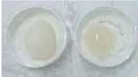
Fig.46: collagen+gelatine+alginate blend. Samples used for swelling, degradation and dehydration test.
