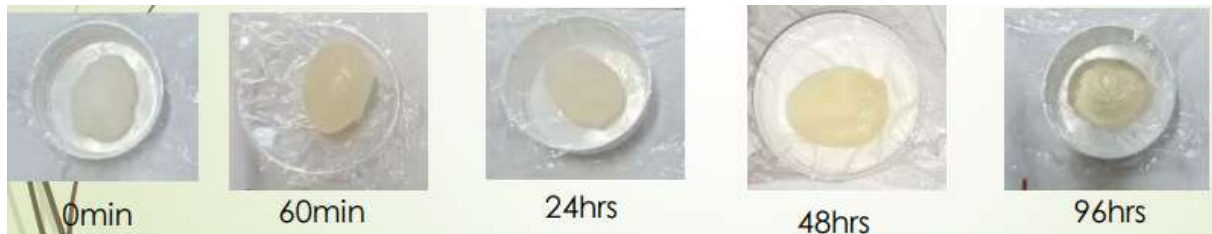
Fig. 47: collagen_gelatine_alginate blend. Samples used for swelling and dehydration tests, weighted at 0, 1, 24, 48 and 96 hours (the results are reported in the Table VI and Table VII above).
