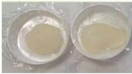
Fig.43: collagen + alginate blend. Samples used for swelling, degradation and dehydration tests.
