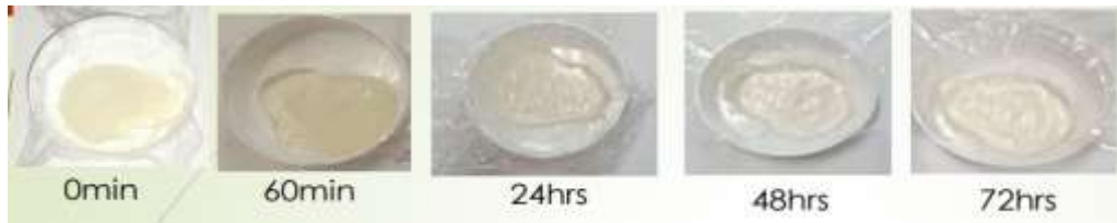
Fig. 44: collagen + alginate blend. Samples used for swelling and dehydration test weighted at 0, 1, 24, 48 and 72 hrs (the results are reported in the Table IV and Table V above).
