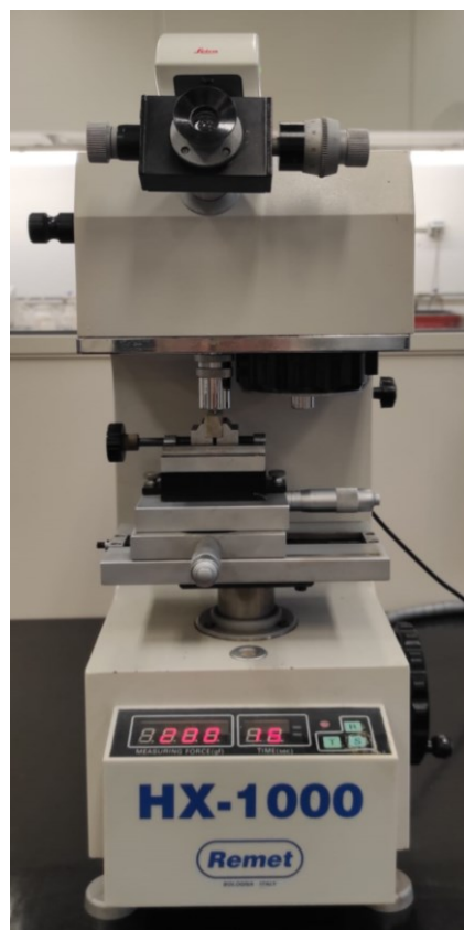
Figura 52. Microdurometro Vickers Remet HX-1000
