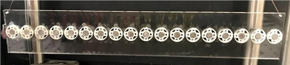
Figure 2. 17: The strip with 18 resonators.
