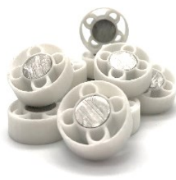
Figure 2. 16: 3D printed resonators with the inner steel mass inserted.
