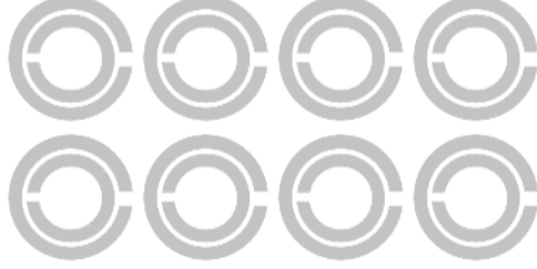
Figure 1.3: Lattice of split ring resonators working as a MNG metamaterial
