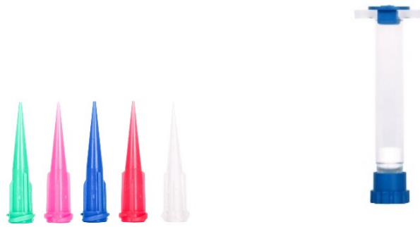
Fig. 21. Bioprinter tools. On the left sterile standard conical bioprinting nozzles, in the order Green-18G, Pink-20G, Blue-22G, Red-25G, Clear-27G, while on the right empty 3 mL pneumatic cartridge [53].
