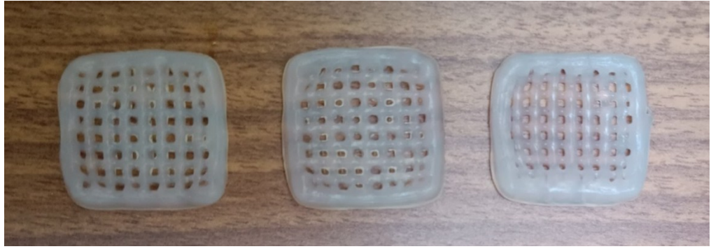
Fig. 43. Three rectilinear scaffolds (20x20x3 mm, 15% infill) realized with the same bioink, 2.5/4, but crosslinked with different crosslinkers. Respectively, starting from left: \text{CaCl}_2 (80 mM) combined with \text{BaCl}_2 (3 mM), \text{CaCl}_2 (80 mM) and \text{CaCl}_2 (300 mM) solutions.
