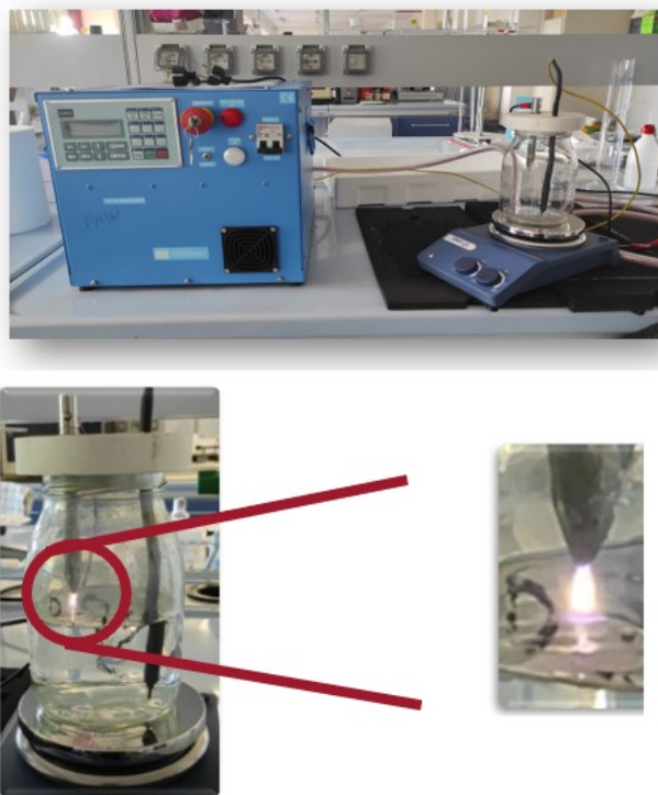
Figure 2-1: Plasma-activated water set-up with corona pulsed discharge
