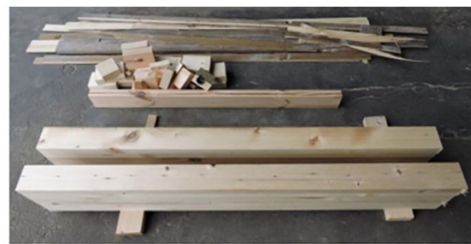
b) Glulam from reclaimed timber
