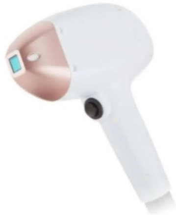
Figure 25. The applicator contains the laser diode emitting visible light at 808 nm [17]. The pink tip is made of anodized aluminium and contains an inorganic glass crystal in the middle. The white part in the user's hands is made of ABS.
