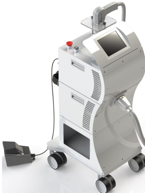
Figure 23. Picture of the laser showing the 3 independent blocks assembled together, including the display and the handpiece [17].
