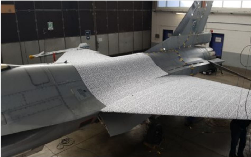
Figure 1.4.: F16 with the speckle pattern placed on top of the wings and on the middle part of the fuselage
