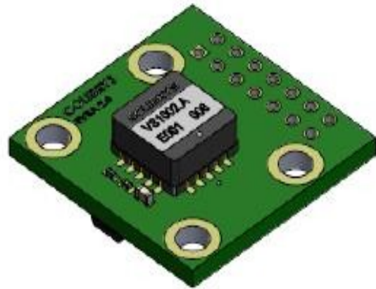
Figura 31: I sensori Safran Colybris VS100 e VS1002
