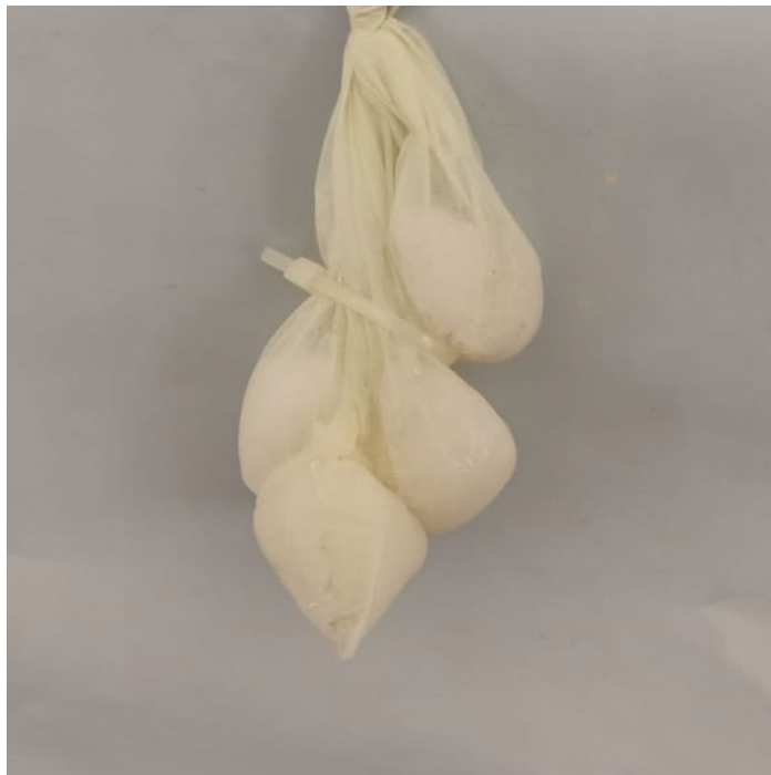
Figure 3. 7: PLA biodegradable plastic bag as an exchange membrane for NaCl Salt.
