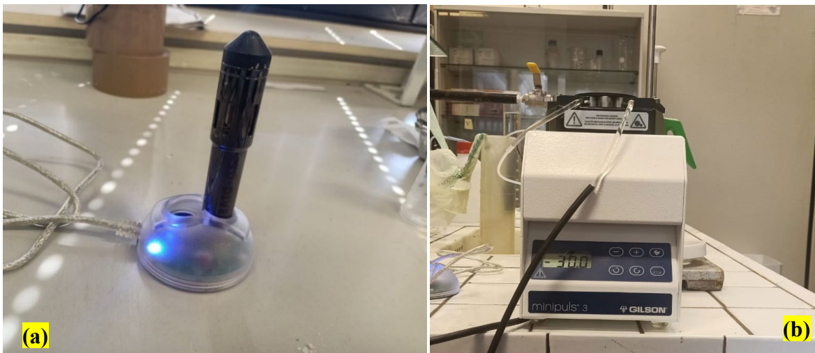
Figure 3. 8: (a) Data logger used in outlet of the tank, (b) Peristaltic pump (MINIPULS® 3 Gilson)
