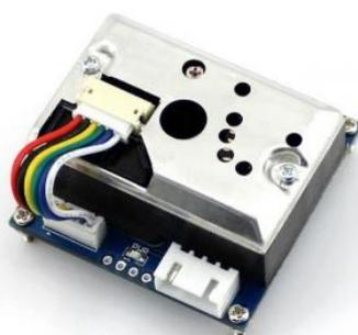
**FIGURA 16.** GP2Y1010AU0F (Dust Sensor)
