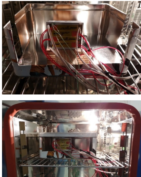
Figure3.43: Thin film insert positioning inside the test chamber.
