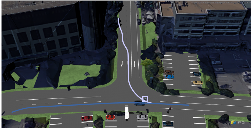
Figure 6.22: Scenario 4: vehicle(blue) hits the cyclist (white boundaries), during the turn left maneuver.
