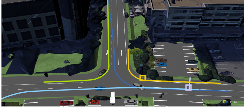
Figure 6.31: Scenario 6: the LandRover TO1 (blue), after overtaking the black vehicle (green), turns right and hit the pedestrian (red). The last vehicle and the cyclist keep their lanes and hit the pedestrian respectively at t = 3.7s and t = 9.15s .
