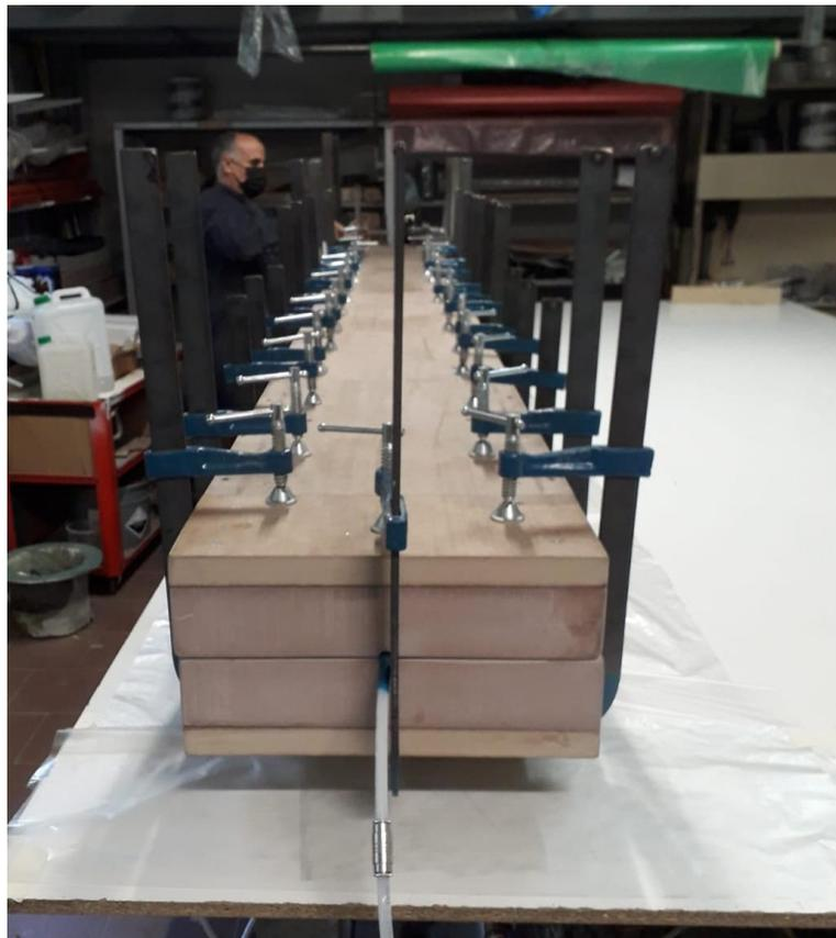
Figura 69: PRESSATURA DOPO INCOLLAGGIO
