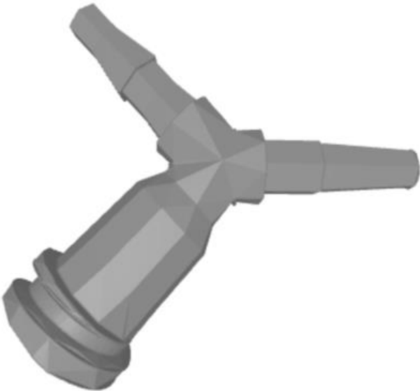
Fig. 16: Device for the creation of the coaxial catheter.
