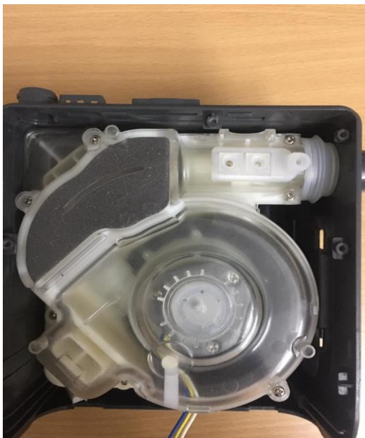
Fig.3.8. Blower setup with BLDC board
