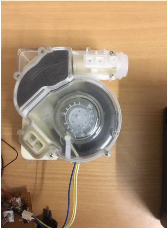
Fig.3.8. Blower setup with BLDC board
